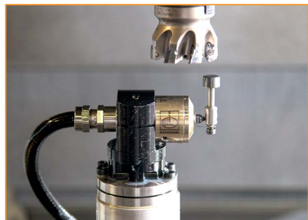
Automatic tool measurement using the TS27R
